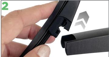
Gently rock the blade and lift it upwards so it disengages from the arm.
