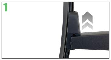
Lift the car's rear wiper arm off the rear screen then gently tilt the blade until it is at 90° to the arm.
