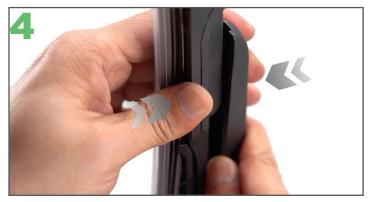
Gently push the Ezywiper blade onto the arm until it locks into place.
