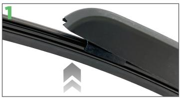
Lift the car's rear wiper arm off the rear screen as far To remove the current wiper blade gently rotate the as it will go.
