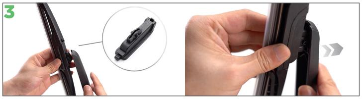
To fit the new Ezywiper blade, align the cross pin on the connector with the grooves on the underside of the arm.
