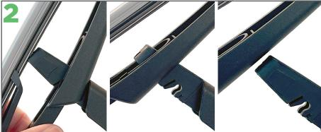
To remove the current wiper blade gently rotate and pull the blade away from the arm until it disengages.
