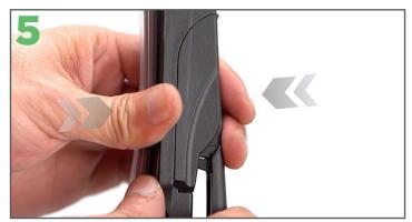
Continue to rotate the blade until it locks into place on the arm.
