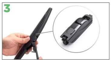
To fit the new Ezywiper blade, align the centre of the Push the blade down and rotate it so the connector's connector's cross pin with the hook on the arm.
