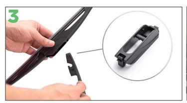
To fit the new Ezywiper blade, align the centre of the Push the blade down so the connector's cross pin fits connector's cross pin into the hook on the arm.
