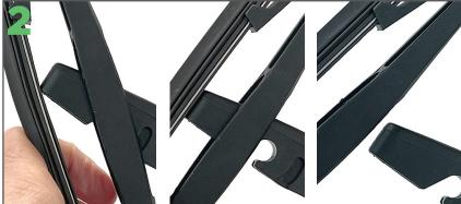
To remove the current wiper blade rotate the end of the blade away from the arm until it disengages.
