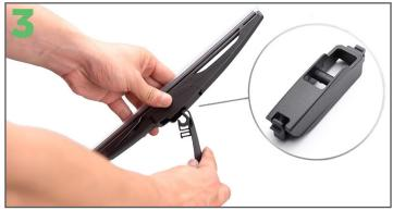
connector's cross pin into the hook on the arm.
