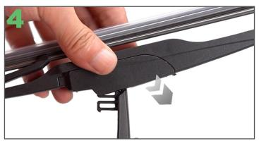
To fit the new Ezywiper blade, align the centre of the Push the blade down so the connector's cross pin fits into the hook on the arm.
