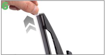
Don't forget to remove the protective sleeve from the Ezywiper blade before placing the arm back on the rear screen.
