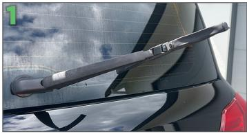
Lift the car's rear wiper arm off the rear screen as far To remove the current wiper slowly rotate the wiper as it will go.
