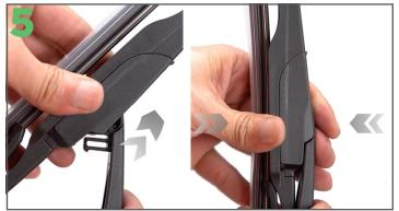
Rotate the blade towards the arm until it locks into place.
