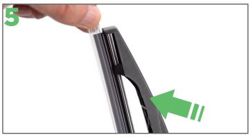
Remove the protective sleeve from the Ezywiper blade before placing the arm back on the rear screen.
