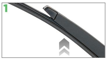
Lift the car's rear wiper arm off the rear screen as far To remove the current wiper blade push the button as it will go.
