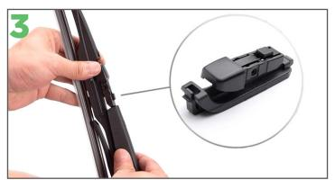
To fit the new Ezywiper blade, line the wiper blade up Push the button on the connector as you firmly slide with the arm.
