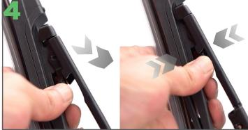
Rotate the blade towards the arm while pinching the side tabs until the blade locks into place.
