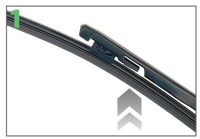
Lift the car's rear wiper arm off the rear screen.
