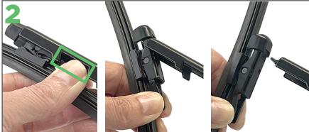
To remove the current wiper blade pinch the tabs on both sides of the connector and rotate the wiper away from the arm.
