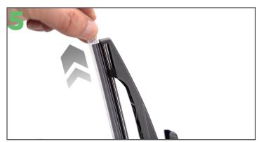
Don't forget to remove the protective sleeve from the Ezywiper blade before placing the arm back on the rear screen.
