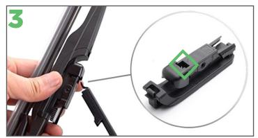
To fit the new Ezywiper blade, insert the tab (see inset) at the top of the wiper into the arm.
