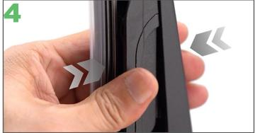
Gently push the Ezywiper blade onto the arm until it locks into place.
