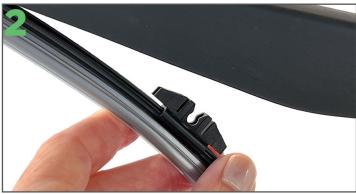
To remove the current wiper blade gently rotate the blade away from the arm until it disengages.
