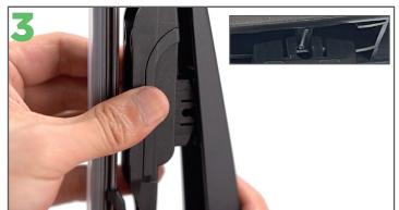
Next, remove the new Ezywiper blade from its packaging. To fit the new Ezywiper blade, align the blade with the arm (see inset).
