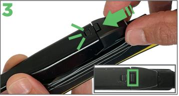
Push the clip (see inset) then slide the blade in until it Remove the protective sleeve from the Ezywiper locks into place.
