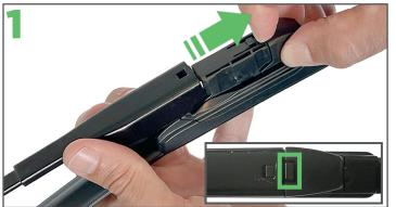
To remove the current wiper blade push the clip down (see inset) and slide the blade away from the arm.
