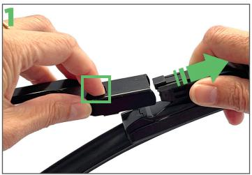
There are two common sizes of push button arm for your vehicle - either 16 millimetres or 19 millmetres wide. First we'll figure out what one your car has. Start by removing the current wiper blade by pushing the button down and sliding the blade away from the arm.
