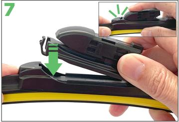
Take your chosen B5 or B2 adaptor and fit the back of it into the wiper mount then guide the front end in. It will click into place (see inset).
