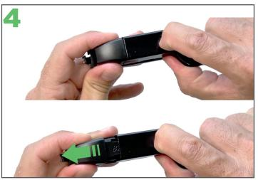
Once you've chosen your adaptor remove it from the arm so it can be fitted to the new Ezywiper blade.
