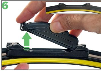
Push the clip so the adaptor releases and can be removed (see the inset for what the wiper looks like once the adaptor is gone).
