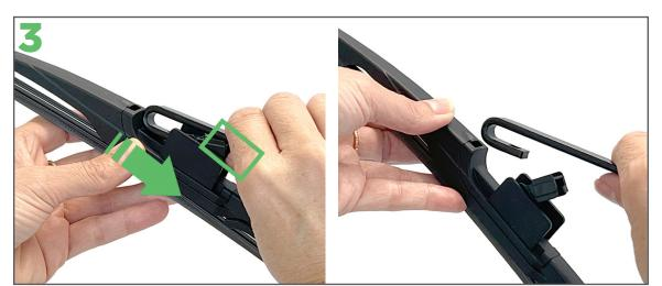
To remove the current wiper, push the tab and slide the wiper until it disengages from the arm.
