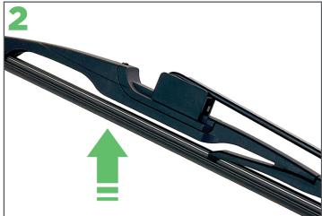
Lift the car's rear wiper arm off the rear screen.
