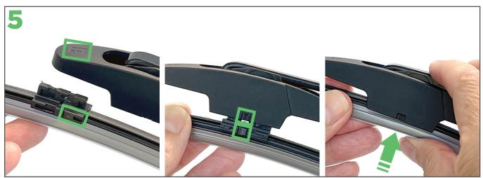
To fit the Ezywiper blade, check the arrows on the blade mount and adaptor are pointing in the same direction.
