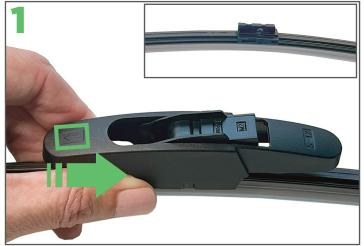
Take the new Ezywiper blade from its packaging. Remove the adaptor on the Ezywiper blade by first locating the arrow at the top of the adaptor, then gently pushing in the opposite directon until the adaptor disengages (see inset for what the wiper looks like once the adaptor is removed).
