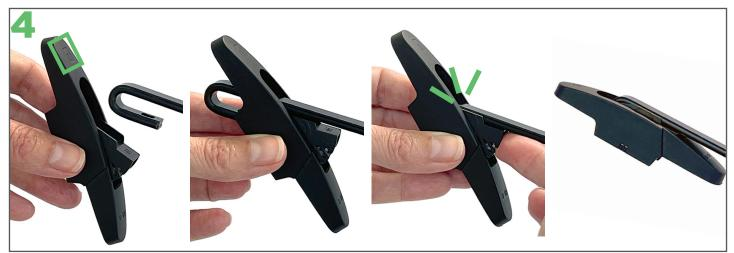
Next, fit the Ezywiper adaptor onto the car's wiper arm. Have the arrow end of the adaptor at the front of the arm. Tilt the tabs inside the adaptor then fit the adaptor onto the arm. Gently slide the adaptor onto the arm so the adaptor locks into place.
