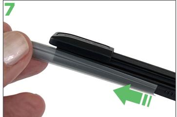
Don't forget to remove the protective sleeve from the Ezywiper blade before placing the arm back on the rear screen.
