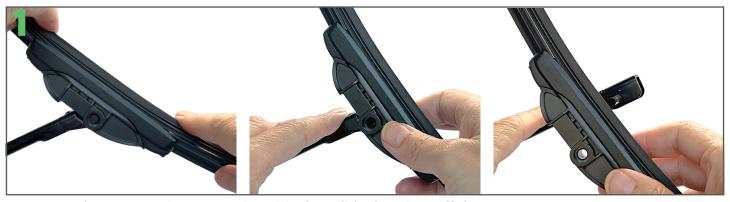
To remove the current wiper, rotate it to 90° then slide the wiper off the arm.
