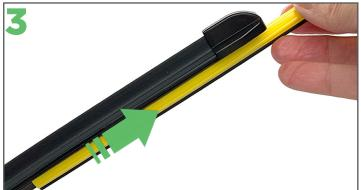
Remove the protective sleeve from the Ezywiper blade then place the arm back on the windscreen.
