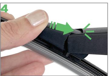
Gently push the Ezywiper blade onto the arm until it locks into place.
