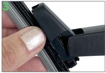
To fit the new Ezywiper blade, hold it at 45° to the arm and place it in position.
