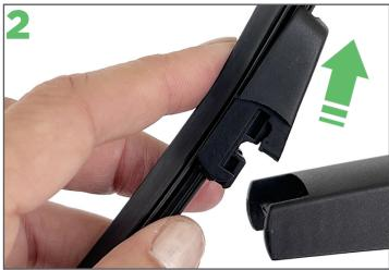
Gently rock the blade and lift it upwards so it disengages from the arm.
