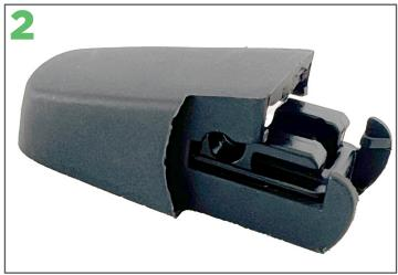
Select the V-Notch adaptor from the bag of adaptors supplied with the blade.
