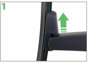
Lift the car's rear wiper arm off the rear screen then gently tilt the blade until it is at 90° to the arm.
