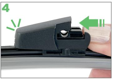
Slide the adaptor in the direction of the blade mount's arrow until the adaptor clicks into place.
