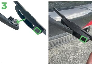
To fit the new Ezywiper blade, align the centre of the Remove the protective sleeve from the Ezywiper adaptor's cross pin into the space on the arm. Make sure the adaptor's arrow is pointing outwards from the arm.
