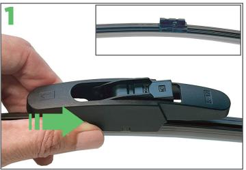
Remove the new Ezywiper blade from its packaging. Your car's wiper arm needs a different adaptor than the one on the Ezywiper blade. To remove the adaptor, locate the arrow at the top of the adaptor, then gently push in the opposite direction until the adaptor disengages (see the inset for what the wiper looks like once the adaptor is removed).
