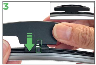
Check the arrows on the blade mount and adaptor are pointing in the same direction.
