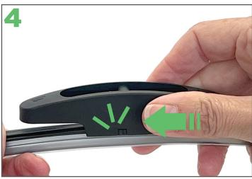
Slide the adaptor in the direction of its arrow until it locks into place.
