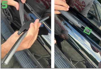
Rotate the blade and place the wiper back on the windscreen.
