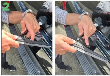
Slowly rotate the wiper while pulling it away from the arm until it disengages.
