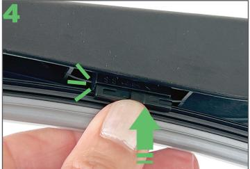
Gently push the Ezywiper blade onto the arm until it locks into place.
