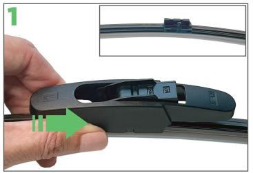
Remove the new Ezywiper blade from its packaging. Your car's wiper arm needs a different adaptor than the one on the Ezywiper blade. To remove the adaptor, locate the arrow at the top of the adaptor, then gently push in the opposite direction until the adaptor disengages (see the inset for what the wiper looks like once the adaptor is removed).
