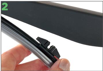
To remove the current wiper blade gently rotate the blade away from the arm until it disengages.
