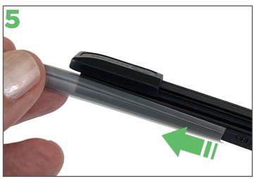
Don't forget to remove the protective sleeve from the Ezywiper blade before placing the arm back on the rear screen.
