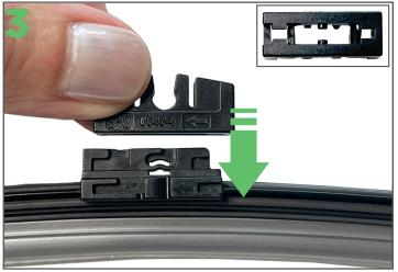
The bottom of the adaptor has a slot that fits over the mount on the blade (see inset).
