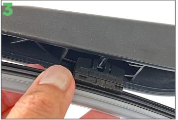
To fit the new Ezywiper blade, align the blade with Gently push the the arm. The arrows on the mount and adaptor point locks into place. to the front of the arm.
