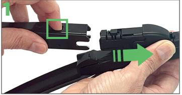
To remove the current wiper blade push the button down and slide the blade away from the arm.
