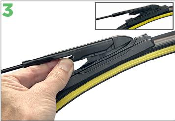
Rotate the blade while pinching the side tabs until the blade locks into place (see inset).
