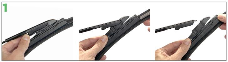
To remove the current wiper blade pinch the tabs on both sides of the connector and rotate the wiper away from the arm.
