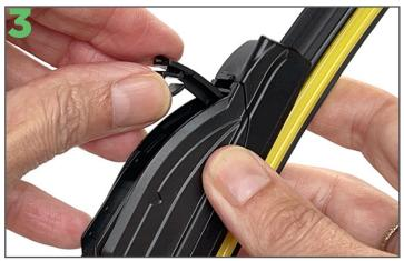
Next, remove the new Ezywiper blade from its packaging. Open the tab on the wiper's adaptor.
