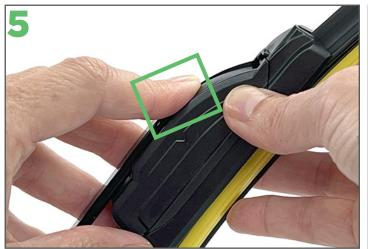
Close the tab on the adaptor and check the blade is securely fitted.
