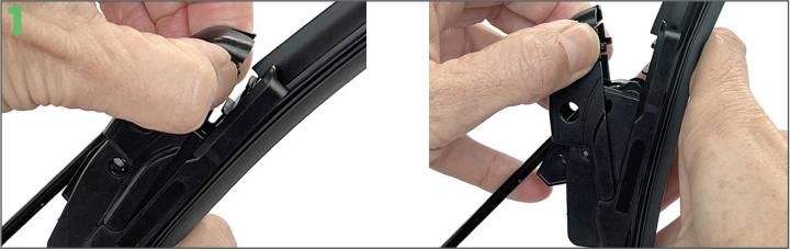
To remove the current wiper blade, open the cap on the top of the blade, then rotate the blade to 45°.
