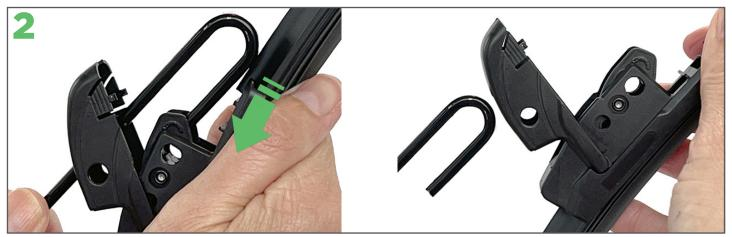
Gently pull the wiper blade down until it disengages from the arm. You may need to press a tab. The blade can then be removed from the arm.
