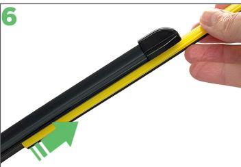
Remove the protective sleeve from the Ezywiper blade before placing the arm back on the windscreen.
