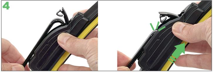
Place the wiper into the arm and gently slide the blade up until it clicks into place.
